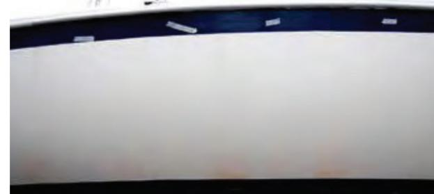
The front and middle of the hull after the test: there's an obvious difference between areas which had been treated and those which hadn't
